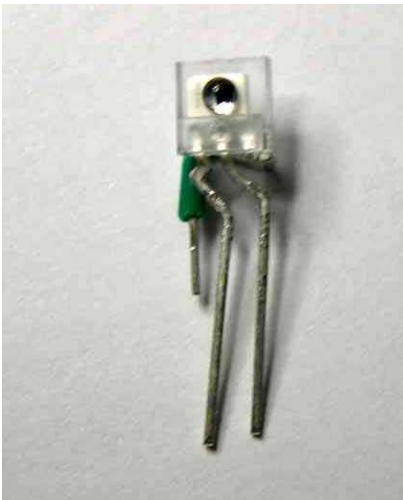
8A. TAOS TSL12S-LF FRONT view, pin 3 is bent around to connect as pin 1, other pins take new positions.
