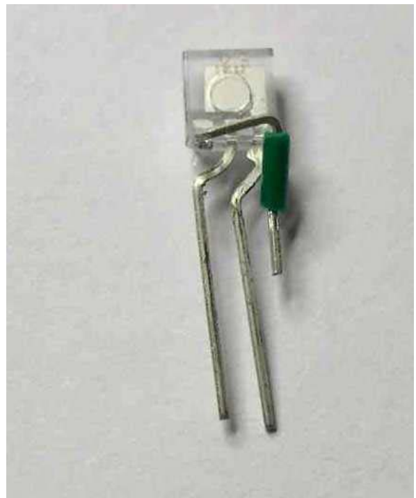
8B. TAOS TSL12S-LF rear view, pin 3 bent behind with insulator to ensure no shorts
